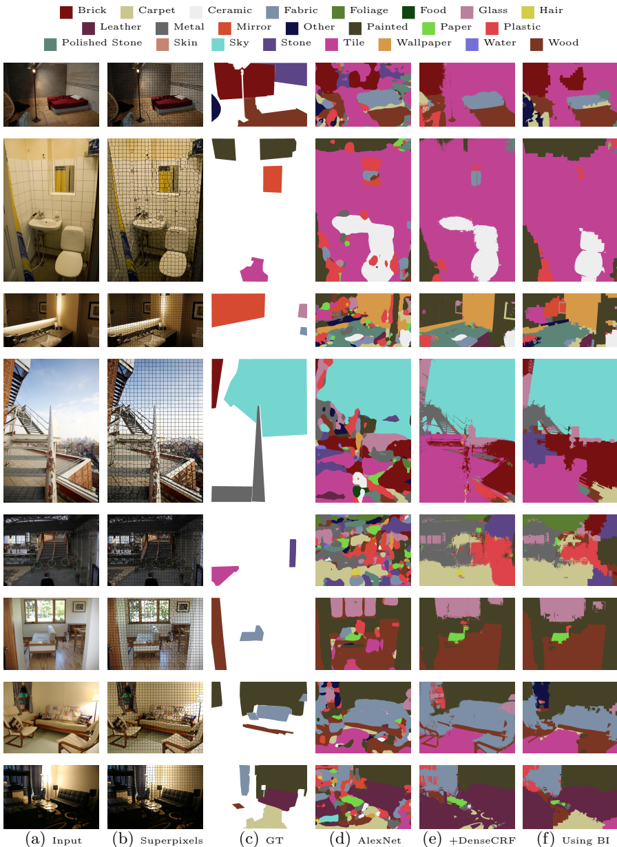
Fig. 2. Material Segmentation. Example results of material segmentation. (d) depicts the AlexNet CNN result, (e) CNN + 10 steps of mean-field inference, (f) result obtained with bilateral inception (BI) modules ( BI_7(2)+BI_8(6) ) between FC layers.
